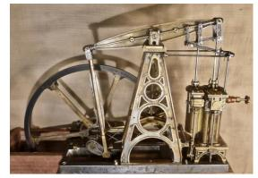
what is concealed inside the castings. The model air pump incorporates lift valves that use chamois leather as the valve rather than rhinoceros hide or latex rubber as in the original. The engine was made by Wentworth and Sons in Wandsworth, and there is a sister engine in the former *Young's* Ram brewery in London, which closed in 2006.
